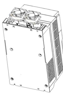
Step 3 Install a new fan in the VFD in the reverse steps. Assemble the VFD. Ensure the air direction of the fan is consistent with that of the VFD (blowing upwards).
