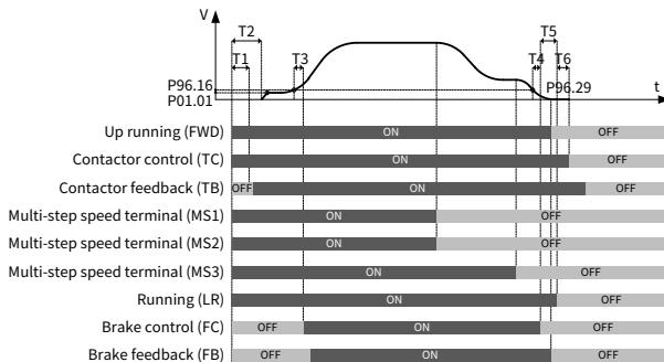
1. After receiving the upward running command FWD and speed commands MS1–MS3 from the controller, the VFD sends the contactor actuation command and outputs the running signal.
