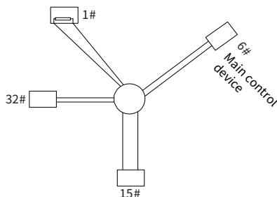
Use shielded cables, if possible, in multi-device connection. The baud rates, data bit check settings, and other basic parameters of all the devices on the RS485 line must be set consistently, and addresses cannot be repeated.
