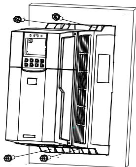
Step 2 Fix the VFD on the wall or mounting plate, and tighten the screws on the wall or mounting plate.
