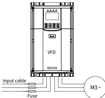
➤**Note:** Select the fuse according to section [E.2 Breaker and electromagnetic contactor](#).
