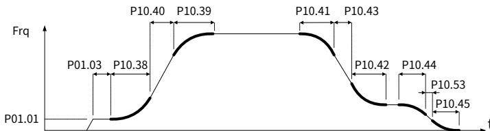
Figure 6-6 S-curve parameter adjustment
