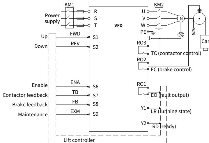
The maintenance running is the same as the normal timing sequence. The maintenance ACC/DEC is linear. The maintenance speed is set by P10.46.
