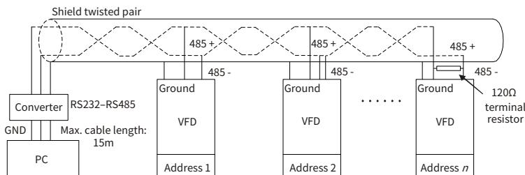
Figure 7-5 shows the start connection diagram. When this connection mode is adopted, each of the two devices that are farthest away from each other on the line must be configured with a terminal resistor (in this figure, the two devices are devices 1# and 15#).
