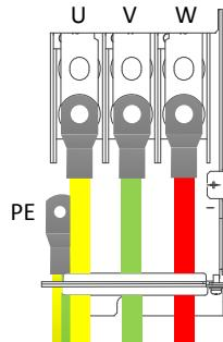
Step 3 Connect optional parts such as the braking resistor that carries cables to designated positions. For details, see section [4.2.4 Main circuit wiring diagrams](#).
