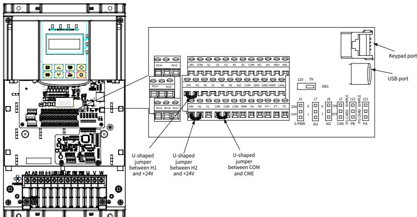
Use the jumper J1 to set the NPN /PNP mode for S terminal inputs. NPN internal mode is adopted by default.
