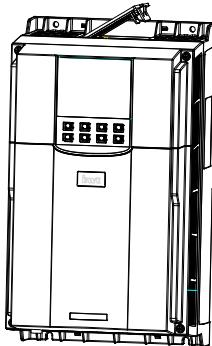
Step 2 Lift the fan upward, and remove the fan connection terminal.
