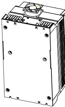
Step 3 Install a new fan in the VFD in the reverse steps. Assemble the VFD. Ensure the air direction of the fan is consistent with that of the VFD (blowing upwards).
