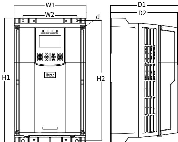
Table D-1 Dimensions and mounting hole size of 2.2–15kW VFD models
