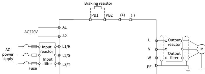
**Note:** The fuse, braking reactor, input reactor, input filter, output reactor, and output filter are optional parts. For details, see [Appendix E Peripheral accessories](#).
