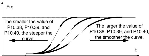
The above figure describes the S-curve parameter adjustment during the acceleration segment, in which the S curve changes sharply when the time parameter decreases while the S curve changes slightly when the time parameter increases. The S-curve parameter adjustment principle during the DEC segment and stop segment are similar to that during the ACC segment.
